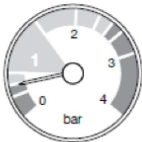
If the water pressure drops below 1.0 bar you need to repressurise your central heating system. This is a simple maintenance job that you should be able to do yourself quite easily, and is best done when the system is cold.
