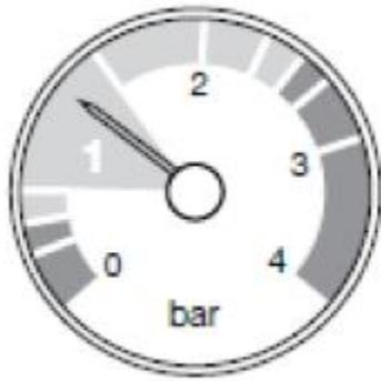
Heat only (or regular) boilers installed on a pressurised system will have a pressure gauge installed in the pipework.
